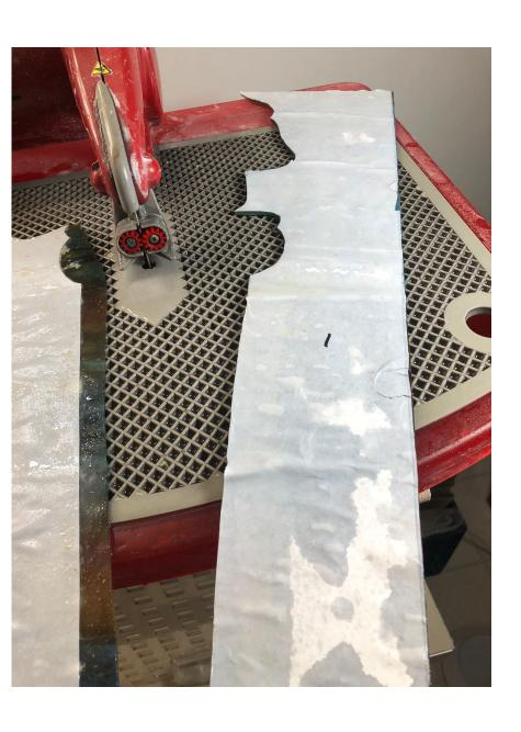
Using a wet ring saw to cut out the more intricate bits
